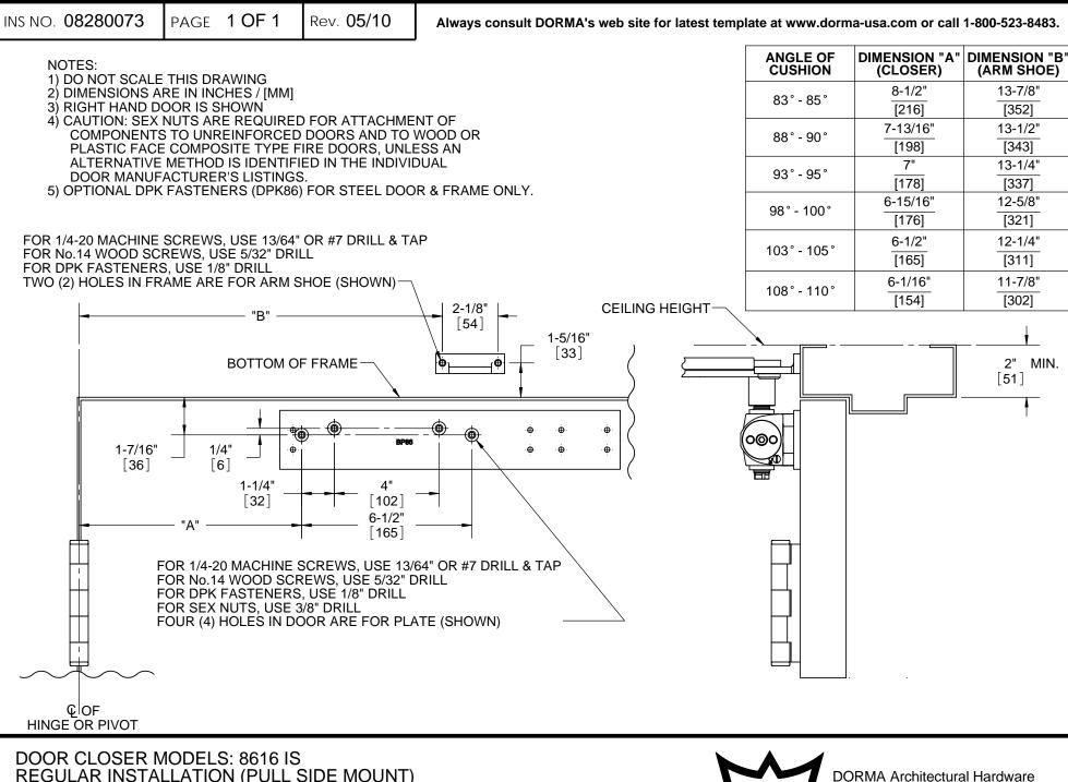
REGULAR INSTALLATION (PULL SIDE MOUNT) WITH PLATES BP86 & BP86FC INTEGRA CUSHION ARM
