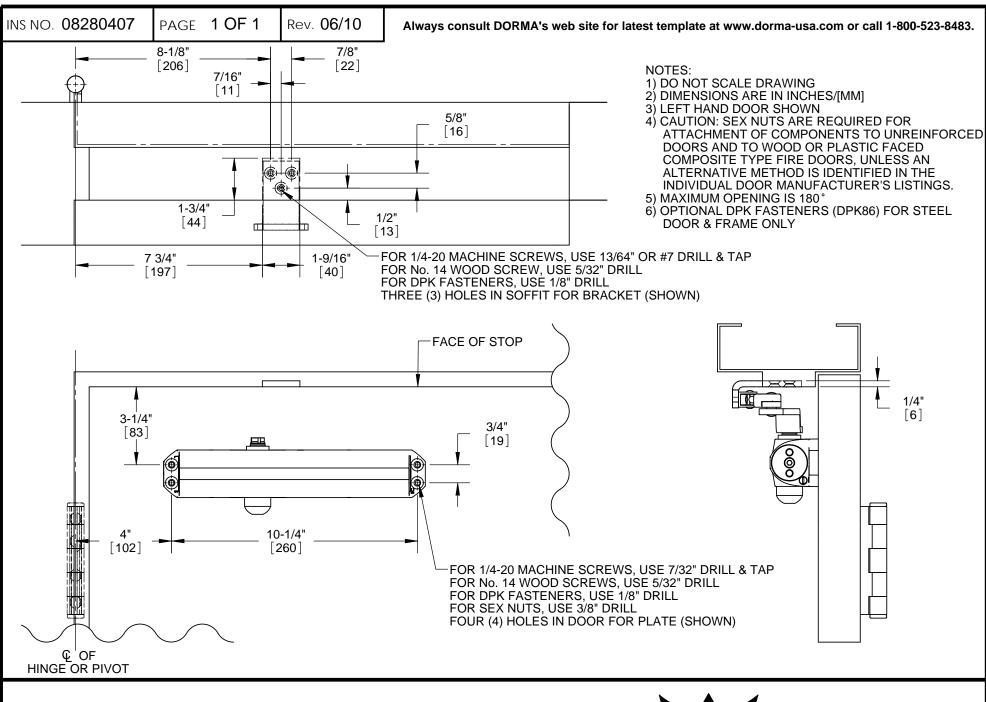
DOOR CLOSER MODELS: 7414 & 7436 ARP x MJ PARALLEL ARM INSTALLATION (PUSH SIDE MOUNT)
