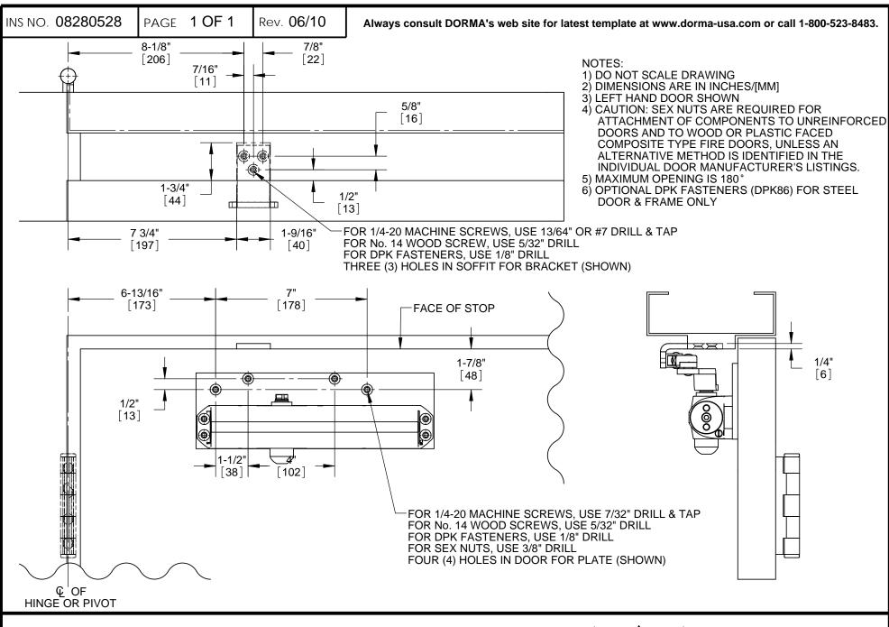
DOOR CLOSER MODELS: 7414 & 7436 ARP x MJ PARALLEL ARM INSTALLATION (PUSH SIDE MOUNT) WITH PLATES DP74, DP86 & DP86FC
