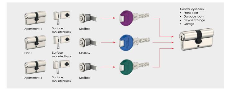
With the special **administrator master key system**, the main areas of several properties (i.e. several locking systems) in different locations can be closed with only one key (administrator key).
