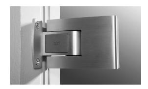
TENSOR double-acting hinges enable tempered glass doors to return to their desired closed position without requiring concealed floor or overhead closers. TENSOR hinges can be mounted directly to the masonry or to a non-recessed frame. In the case of a "glass-to-glass" model, the double-acting door is hung from the sidelite.
