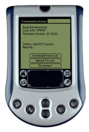
Once the Download has completed, a message will be displayed indicating that the download is complete. The lock data has been received at the M-Unit and is ready to be transferred to the PC.
