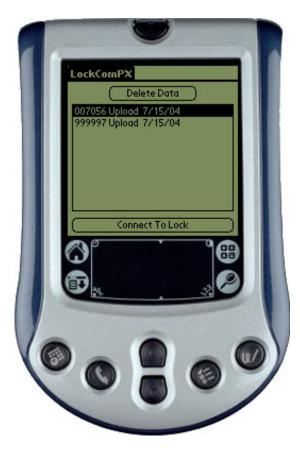
7. Select the appropriate lock "upload" entry and tap on **Connect to Lock.**
