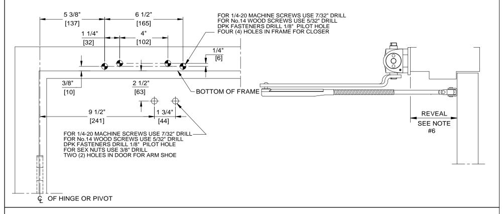
DOOR CLOSER MODELS: 7414, 7436 ARJ (NHO) TOP JAMB INSTALLATION (PUSH SIDE MOUNT) WITH PLATES BP74, BP86, BP86FC
