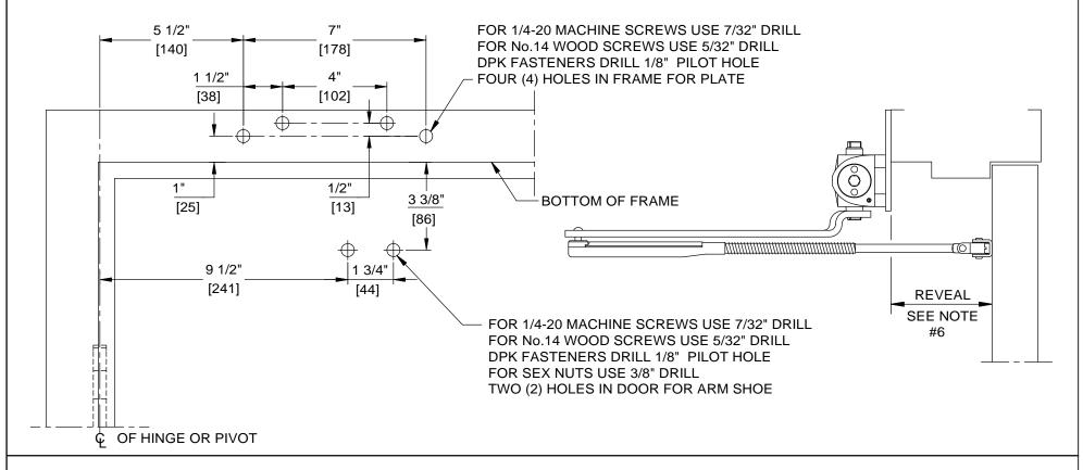
DOOR CLOSER MODELS: 7414, 7436 ARJ (NHO) TOP JAMB INSTALLATION (PUSH SIDE MOUNT) WITH PLATES DP74, DP86
