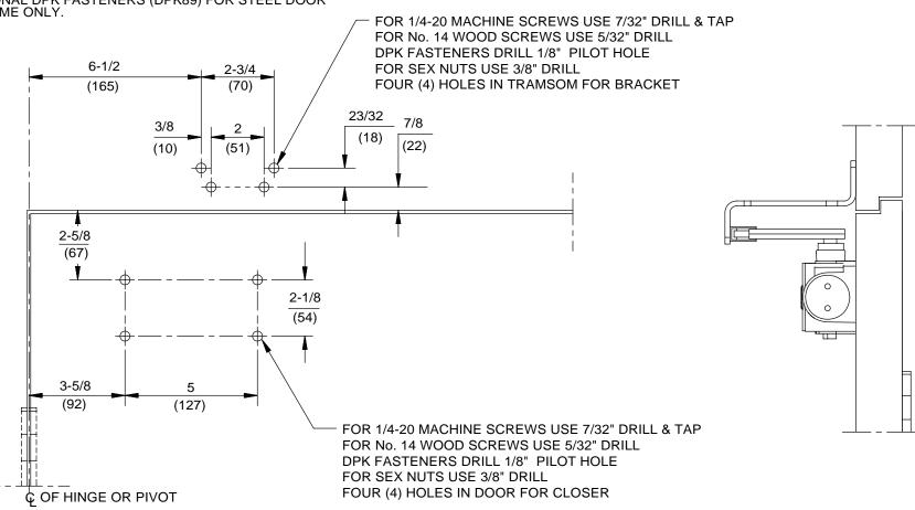
DOOR CLOSER MODELS: 8916, 8956 AF89 PH or PFT BRACKET PARALLEL ARM FLUSH TRANSOM INSTALLATION (PUSH SIDE MOUNT)
