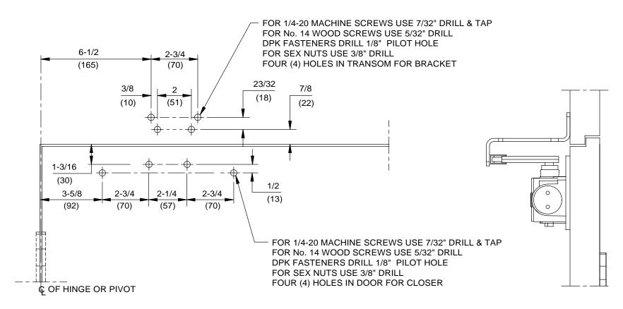
DOOR CLOSER MODELS: 8916, 8956 AF89 PH or PFT BRACKET PARALLEL ARM FLUSH TRANSOM INSTALLATION (PUSH SIDE MOUNT) WITH PLATE DP89
