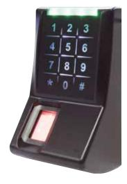
accommodates up to eight readers and 1,000 users or 500 finger template pairs per AM300. If access control requirements entail a large number of readers and users, the AR402 combined with Kaba's Access Manager 524 (AM524) and Door Unit (DU) supports up to 24 readers and 6,000 users or 3,000 finger pairs per AM524. With either configuration, the system offers three-factor authentication: biometrics, PIN code, and optional iCLASS® card.
