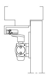
DOOR CLOSER MODELS: 7302 - 7306 ARP x MJ PARALLEL ARM INSTALLATION (PUSH SIDE MOUNT) WITH PLATES DP73, DP86, DP86FC
