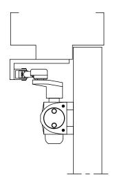
DOOR CLOSER MODELS: 7302 - 7305 ARP x MJ PARALLEL ARM INSTALLATION (PUSH SIDE MOUNT)
