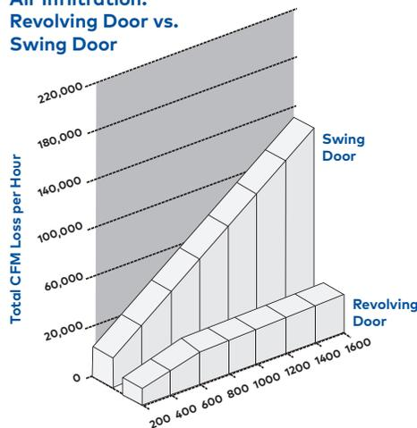
Infiltration rates through a swing door are about 900 cubic feet (25.5 cubic meters) per person for a single-bank entrance, and 550 cubic feet (15.6 cubic meters) per person for a vestibule entrance. But it is only about 60 cubic feet (1.7 cubic meters) per person for a manually operated revolving door, and 32 cubic feet (0.9 cubic meters) per person for an automatic revolving door.
