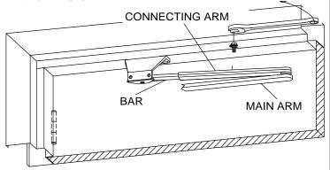
Adjust spring tension, if required, using a 1/4" wrench.
