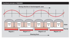
MAGNEO—driven by linear magnetic drive (LMD) technology
