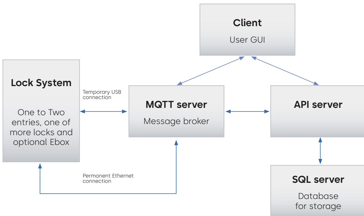
There are two possible connections between the lock system and the local SW. One is direct connection over USB to the entry. This connection must be enabled by an authorized user in the menu selection of the lock. The second connection is from the E-box over Ethernet to the local SW.
