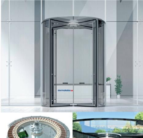
KT FLEX Direct the new electromagnetic direct drive system minimises tolerances and wear. Its gearless power transmission is based on magnetic technology - tested to 2 million cycles. The LED ring in the all-glass revolving doors elegantly highlights the drive and simultaneously provides constant flicker-free illumination of the interior.
