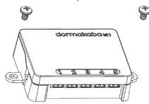
2. Connect each safe lock into the numbered input ports on the Multiplexer (up to 5).
