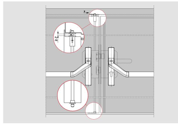
Vertical locking, sheet steel door – For panic exit devices according to EN 1125 a floor keep is necessary (see page 19)
