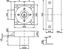
E = Installation depth in mm D = backset (25 mm)
