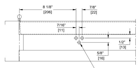
FOR 1/4-20 MACHINE SCREWS USE 7/32" DRILL & TAP \(^1\) FOR No.14 WOOD SCREWS USE 5/32" DRILL DPK FASTENERS DRILL 1/8" PILOT HOLE THREE (3) HOLES IN SOFFIT FOR BRACKET
