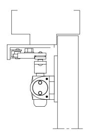
DOOR CLOSER MODELS: 8616 AFP x MJ PARALLEL ARM INSTALLATION (PUSH SIDE MOUNT) WITH PLATES DP86, DP86FC
