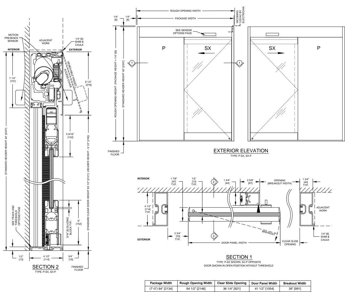
96 1/2" [2451] 42 1/4" [1073] 47 1/2" [1207] 45" [1143] (8'-0") 96" [2438] (Package Width) (Package Width / 2) (Package Width / 2) (Package Width / 2) Width Formulas +1/2" [13] - 1/2" [13] - 3" [76] - 53/4" [146]
