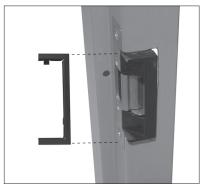
Make sure the Trim Plate series label matches the Strike series you are installing.
