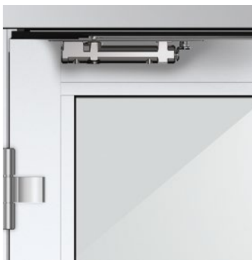
01 Concealed door closer ITS 96 All the single-action sliding panels are equipped with the ITS96 door closer integrated in the door profile and featuring a mechanical hold-open.
