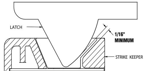
8. Tighten the two mounting screws and check operation. Adjust the horizontal position of electric strike as required.
