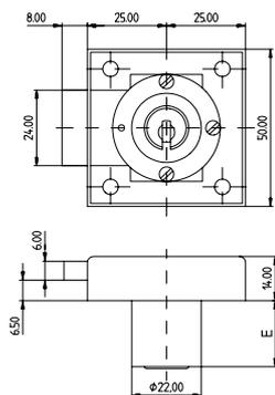
E = Installation depth in mm
