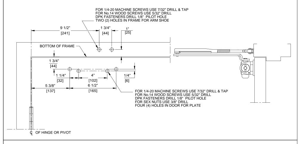
DOOR CLOSER MODELS: 8616 A08 REGULAR INSTALLATION (PULL SIDE MOUNT) WITH PLATES BP86, BP86FC
