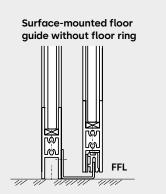
The design of the floor guide depends on the opening width\* and the prevailing on-site conditions and comprises
