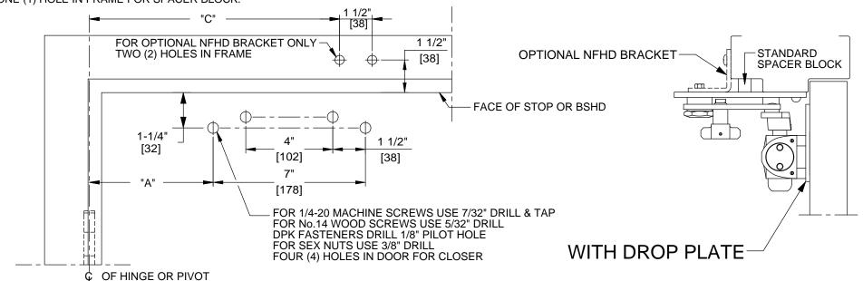
DOOR CLOSER MODELS: 7302 - 7305 SPA, SPAT, SPAK SUPER PARALLEL ARM INSTALLATION (PUSH SIDE MOUNT) WITH PLATES DP73, DP86, DP86FC AND STANDARD SPACER BLOCK OPTIONAL NFHD BRACKET AND BSHD BLADE STOP SPACER BLOCK
