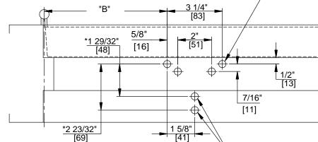
\*IMPORTANT: CHOOSE APPROPRIATE HOLE LOCATION FOR SPACER BLOCK, IN ACCORDANCE WITH FRAME WIDTH. ONE (1) HOLE IN FRAME FOR SPACER BLOCK.
