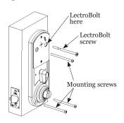
**Warning**: If using a power drill, please be careful not to over-tighten as this could cause damage to the mounting screws and threads.
