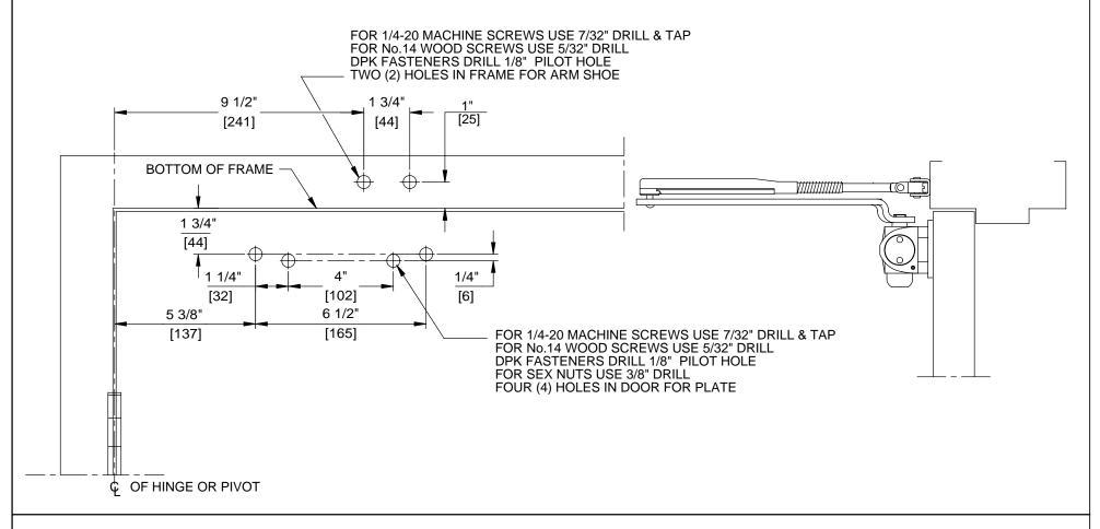
DOOR CLOSER MODELS: 7200/7300 A08 REGULAR INSTALLATION (PULL SIDE MOUNT) WITH PLATES BP73, BP86, BP86FC
