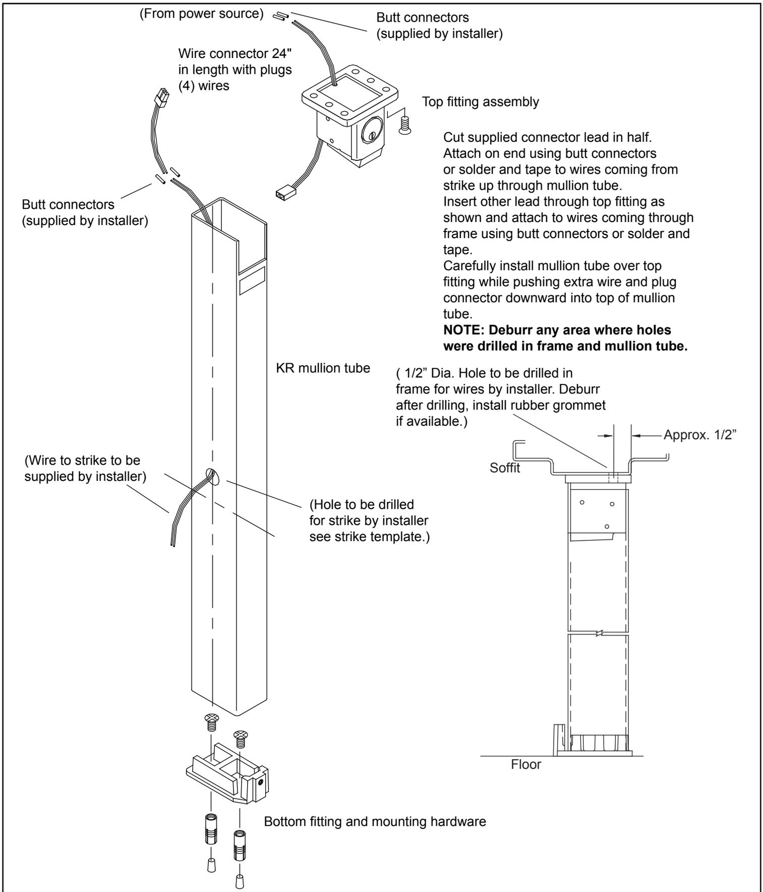
Cut supplied connector lead in half. Attach on end using butt connectors or solder and tape to wires coming from strike up through mullion tube. Insert other lead through top fitting as shown and attach to wires coming through frame using butt connectors or solder and tape. Carefully install mullion tube over top fitting while pushing extra wire and plug connector downward into top of mullion tube.
