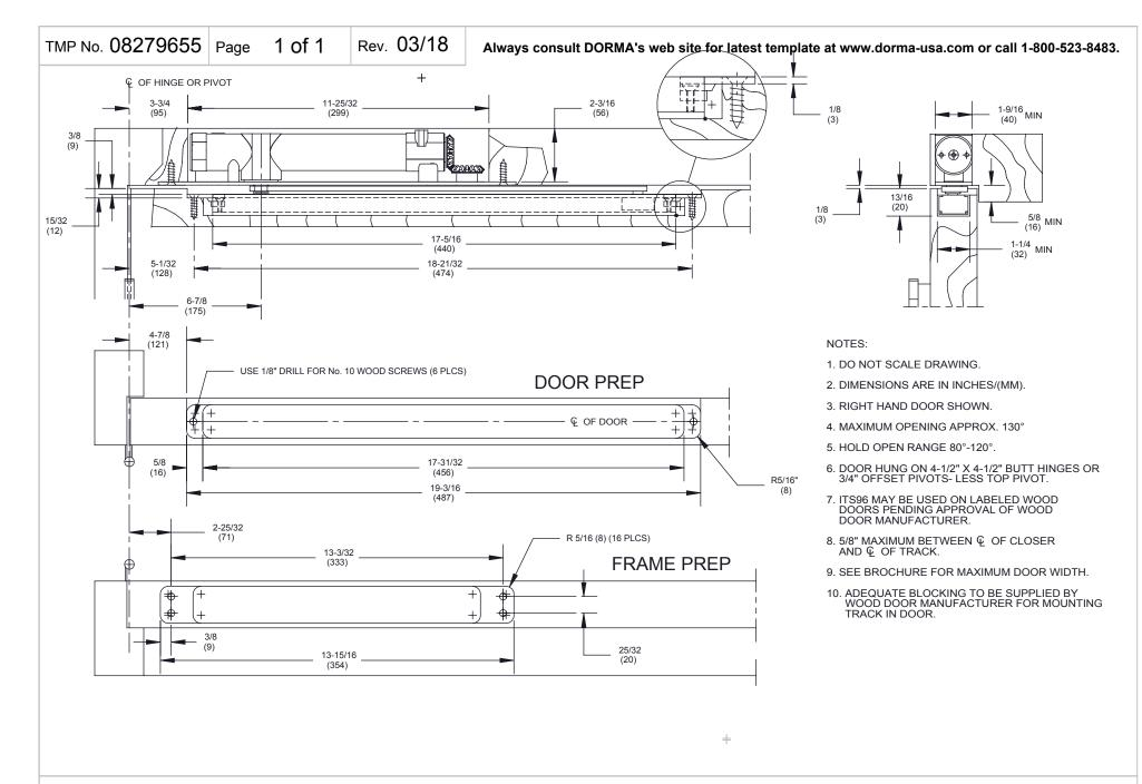
DOOR CLOSER MODEL: ITS9625 INV CLOSER IN FRAME, TRACK IN DOOR WITH ACCESSORY TRACK BRACKETS (WOOD DOOR AND FRAME)
