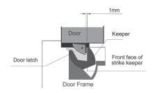
As drawn in the diagram, there should be a 1mm gap between the door latch and the front face of the strike keeper, preventing the door from creating back pressure on the strike keeper when the door is closed. This gap is important to ensure the proper functioning of the strike.
