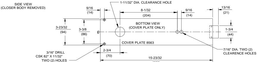
DOOR CLOSER MODEL: RTS SERIES PACKAGE 06, WOOD DOOR AND ALUMINUM FRAME PREPARATION, CENTER PIVOTED 2-3/4" BACKSET, No. 8832 SIDE LOAD ARM, No. 7421 BOTTOM ARM, No. 7471K FLOOR BEARING, No. 8563 COVER PLATE
