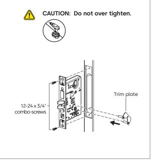
2.2.1 Place outside escutcheon assembly flush against face of door and hold in place.
