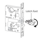
NOTE: Be sure latch foot is raised when reinserting latch.
