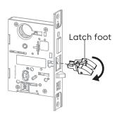
4.2.5 Reinstall latch into lock.
