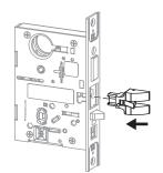
4.2.6 Reinstall latch bolt set screw and tighten securely.
