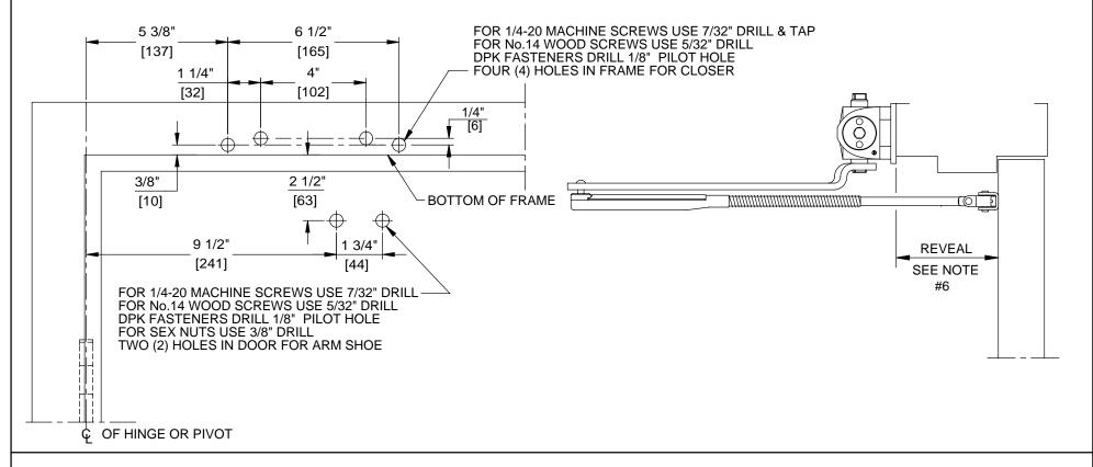
DOOR CLOSER MODELS: 8616 A08J TOP JAMB INSTALLATION (PUSH SIDE MOUNT) WITH PLATES BP86, BP86FC
