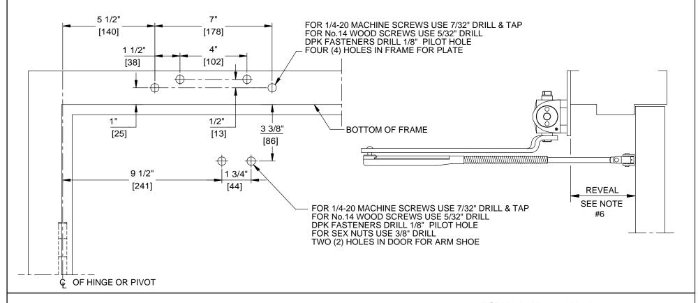
DOOR CLOSER MODELS: 8616 A08J TOP JAMB INSTALLATION (PUSH SIDE MOUNT) WITH PLATE DP86
