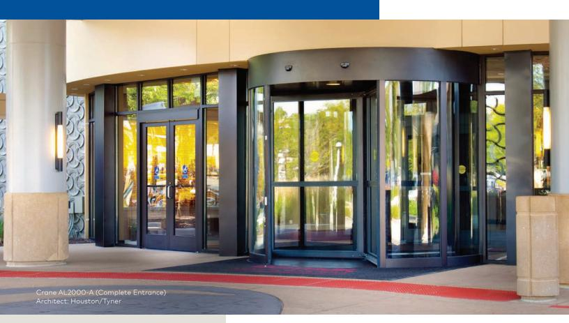
The 2000-A Series features the torquedriven Crane Modular Drive System. The reliable advanced microprocessor control monitors the door and occupants to ensure safe operation.
