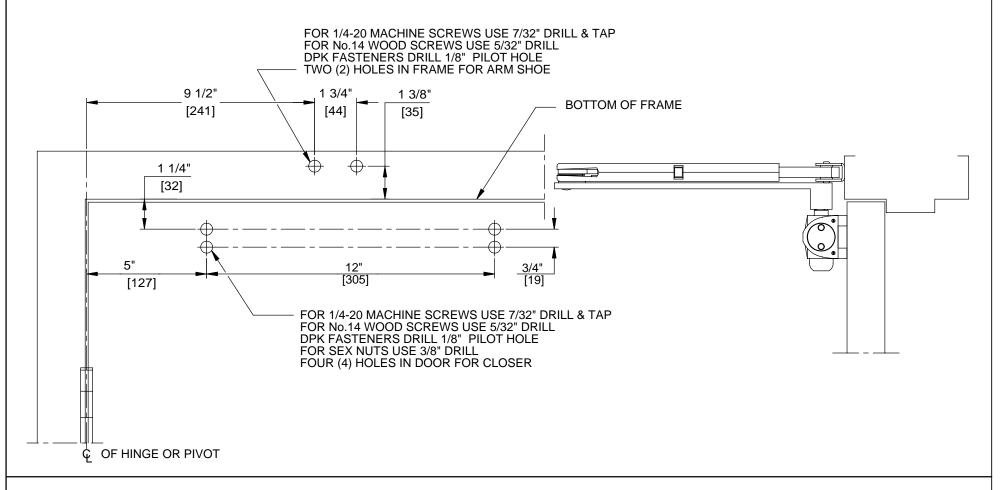
DOOR CLOSER MODELS: 8616 PH REGULAR INSTALLATION (PULL SIDE MOUNT) PLUNGER HOLD OPEN ARM
