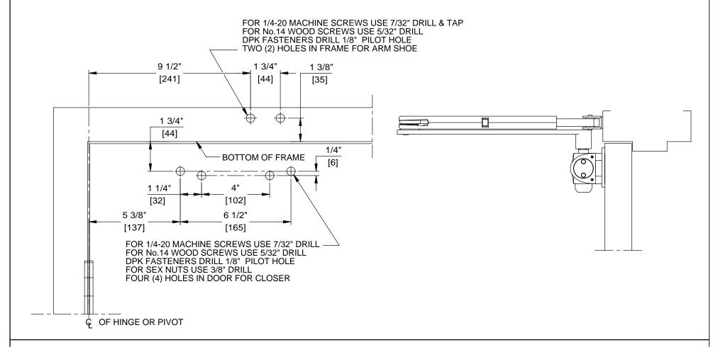
DOOR CLOSER MODELS: 8616 PH REGULAR INSTALLATION (PULL SIDE MOUNT) PLUNGER HOLD OPEN ARM WITH PLATES BP86, BP86FC
