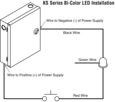
NOTE: To wire LED for green light instead of red light — disconnect red wire from switch point and connect green wire.
