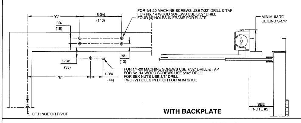
DOOR CLOSER MODELS: 8916 AR STA TOP JAMB INSTALLATION (PUSH SIDE MOUNT) WITH PLATE BP89
