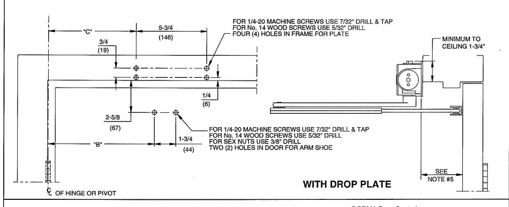
DOOR CLOSER MODELS: 8916 AR STA TOP JAMB INSTALLATION (PUSH SIDE MOUNT) WITH PLATE BP89 DROP
