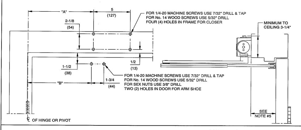
DOOR CLOSER MODELS: 8916 AR STA TOP JAMB INSTALLATION (PUSH SIDE MOUNT)
