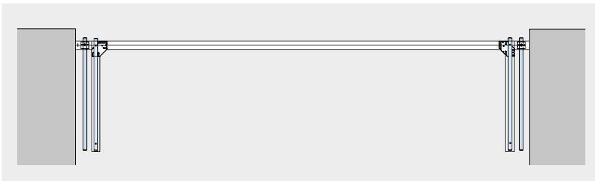
Stacking with one stacking leg for sliding panels in front of the pivoting end panel, single- or double-action, on each side (2 pivoting end panels/2 sliding panels).
