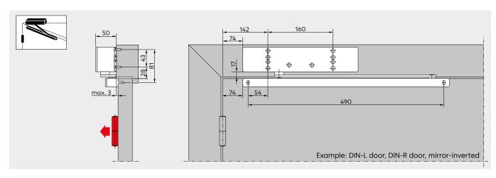
A 180° opening angle is possible in this installation type, provided that the appropriate construction conditions are met.
