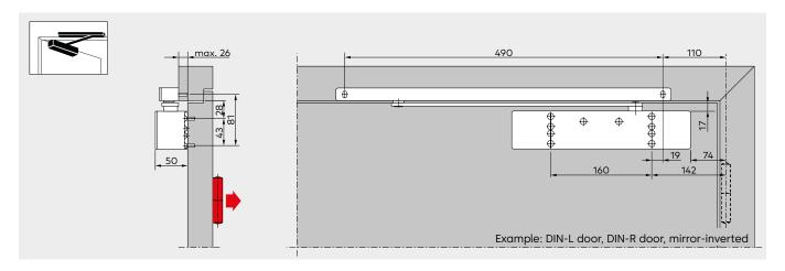
Depending on construction conditions, the door opening angle is limited to approx. 120° to 145°.
