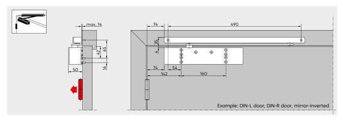
A 180° opening angle is possible in this installation type, provided that the appropriate construction conditions are met. In most cases, the door closer requires a wall recess for that purpose.
