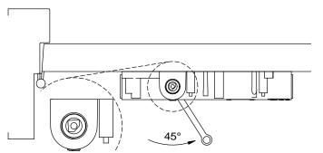
Rotate pinion 45° AWAY FROM HINGE edge of door.
