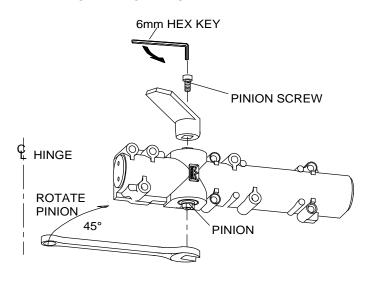
6 Adjust spring tension, if required, using a 1/4" wrench.
