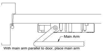
onto top pinion. Fasten securely with pinion
