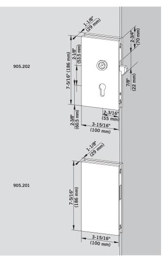
Hook Lock – For sliding doors, prepared for Europrofile cylinder, left hand and right hand, with lock keeper plate, suitable for lever handles with follower
