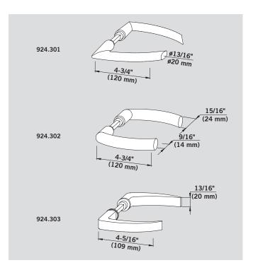
Set of levers Ref. # 924.301 Weight in lb (kg) alumin. 0.77 lb (0.35 kg) brass 2.12 lb (0.96 kg)
