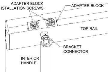
DRS Rails installation instructions for possible adjustments of the top rail. Wind the threaded pivot bracket connector to start thread.
