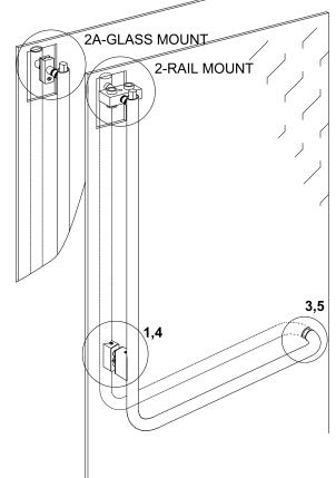
1. To remove the Handle from the board first loosen two flat head socket screws (A) so they protrude approximately 1/4" from Cylinder Housing (B) being careful NOT TO REMOVE them. Push or tap screws flush (C).
