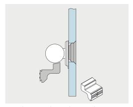
Towards securing the panel an accordant anti-jump device for solid and tubular tracks will be used.
