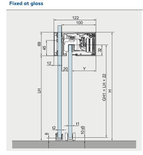
To ensure a correct and aligned mounting of the track rail, a fully supporting fixed panel must be installed.
