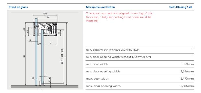
Total height Quantity of drilling distance signed with BA Glass width Н Т Α AB Quantity of drillings LH Clear opening height t1 Glass thickness sliding door Length of track Clear opening width Glass thickness fixed panel (10 – 19 mm) t2 RΑ
