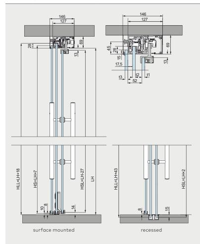
For installation with two door panels and sidelight on one side, fixed at ceiling, optional with DORMO-TION unit. When using a DORMOTION damping unit, we recommend installation of a pull handle.
