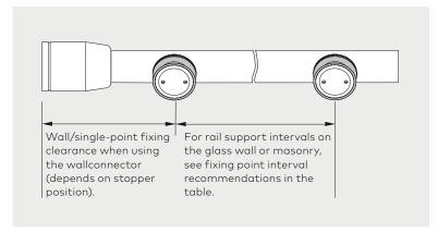
**Caution!** Ensure that the stops/single-point fixings are positioned at locations appropriate to the width of the door.
