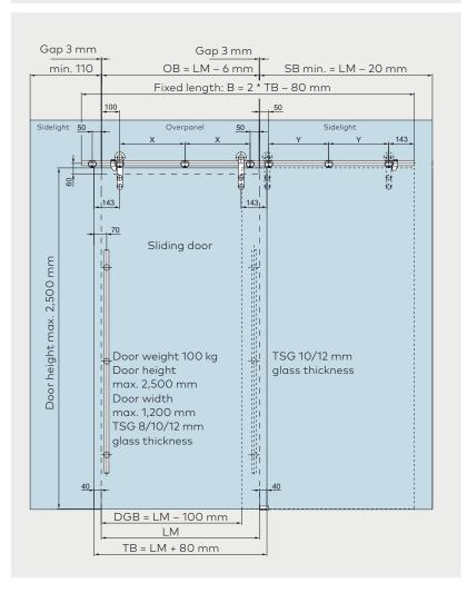
An appropriately dimensioned and torsionally stiff substructure will need to be provided for installation.
