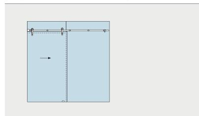
for sliding door 8 – 12 mm glass, fixed element 10 – 12 mm glass
