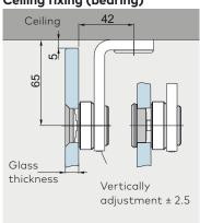
**Note:** Ensure compliance with minimum glass/bore clearances as per glass manufacturer recommendations. Glass preparation with a tolerance of max. ± 0.3 mm is recommended.
