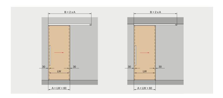
Fixed at wall Fixed at ceiling **Product description** Wood thickness For installation with one door panel 28-50 mm Max. weight of door panels 80 kg Calculation of door height fixed at wall TH = LH - 18 + X mmmax. 3,000 mm Calculation of door height fixed at ceiling TH = H - 76 mm Ξ max. 3,000 mm Calculation of door width A = LW + 60 mmmin. 660 mm max. 2,000 mm \* Timber door 100 mm, solid wood, for attachment to timber adapter.
