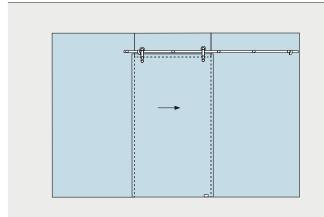
for sliding door 8 – 12 mm glass, fixed element 10 – 12 mm glass
