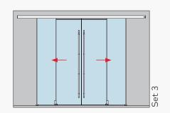
Glass door (8 - 13.5 mm) for the installation at ceiling / with side light (10 - 19 mm) - 2 and 4 panels
