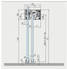
To ensure a correct and aligned mounting of the track rail, a fully supporting fixed panel must be installed.
