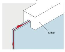
Shrinkage of interlayer (due to temperature and Glass crack pressure variation in long-term usage)
