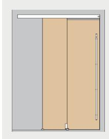
Opening direction left, Closing direction right (DIN right)
