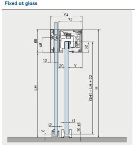
To ensure a correct and aligned mounting of the track rail, a fully supporting fixed panel must be installed.
