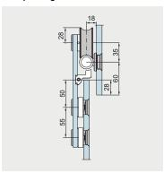
Dimensional data should be regarded exclusively as recommended values. Please remember when designing your system that the positions of the stops and point fixings must not vertically coincide. For spacing/interval recommendations when drilling the track holes, and for requisite dimensions for fixing the track rail, please refer to the table entitled "Recommended distance of the track fixing points".
