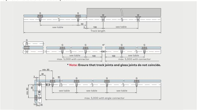
G = Fixing point at glass W = Fixing point at wall K = Connection
