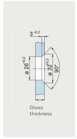
Countersunk bore for countersunk single-point fixings
