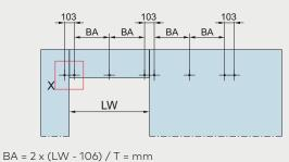
The total quantity of drillings (AB) depends on clear opening width (LW) and determines the final drilling distance (BA).
