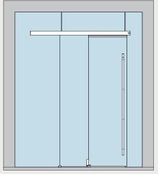
for glass installation, with recessed floor guide profile, 2 panels (left)
