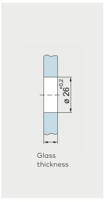
Cylindrical bore for clamping disc single-point fixings
