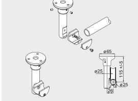
Ceiling retainer double 21.317 for tubular track, carrying function
