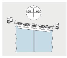
Sliding door gear RS 120 Synchro For 2-panel synchronously opening system,
