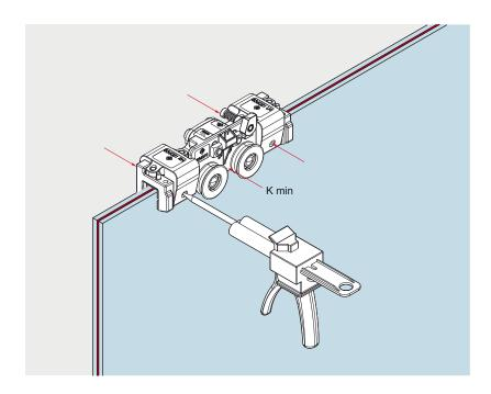
dormakaba Clamp&Glue technology provides the possibility to keep the advantages and – at the same time – to eliminate the potential issues of laminated safety glass. The solution for secure hold of the glass panel only needs a minimum of clamping force at the fittings, without any glass preparation.
