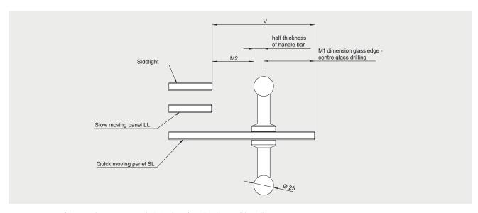
V = Protrusion of the quick-moving panel (SL) when fitted with a pull handle (see Data Sheet 36-747)
