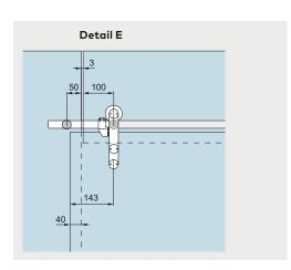
An appropriately dimensioned and torsionally stiff substructure needs to be provided for installation.
