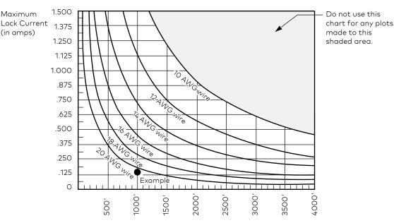
Total Footage of Two Conductor Cables for Lock Circuit (In Feet)
