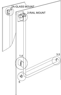
1. To remove the Handle from the board first loosen two flat head socket screws (A) so they protrude approximately 1/4" from Cylinder Housing (B) being careful NOT TO REMOVE them. Push or tap screws flush (C).
