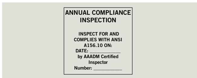
Fig. 4.1.2 Annual compliance inspection labels
